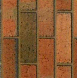
TYPE EX2 IBSTOCK traiford multi rustic Warm tone brick in a stretcher bond pattern or similar approved.
