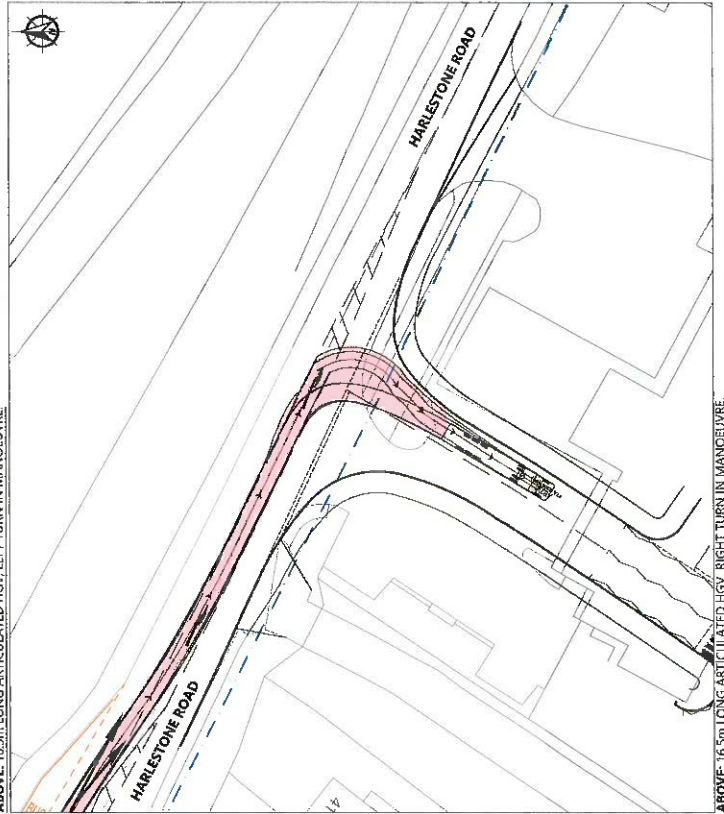
ABOVE: 16.5m LONG ARTICULATED HGV, RIGHT TURN OUT MANOEUVRE
